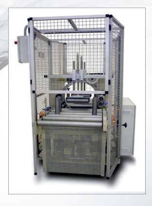
Fully automatic twist wrapping machine for all kinds of profiles and long products in "plug-and-play" design.
