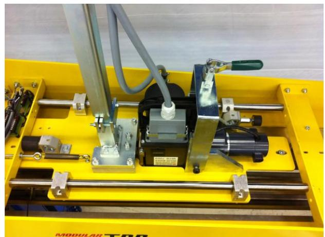
For improved strap tension transmission around the load and a more secure product the MH sealer unit is mounted on a floating head carriage. This ensures consistent and optimum pallet load securement.
