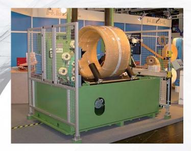
Fully automatic standard universal twist wrapping machine for ring-shaped products ("plug-and-play")
