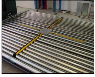
Seen here is the integrated pallet turn-cross located inside the press in the roller conveyor. The maximum pallet load weight which can be handled is 1.500 kg
