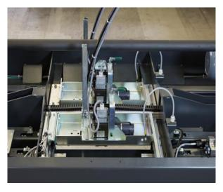
GCU 2800 machine platen showing the modular applicators applying the corrugated straps to the top and the bottom of the load before strapping. The modular MH head design enables modules to be easily accessed for service and maintenance and can be exchanged in less than 2 minutes for maximum machine uptime.
