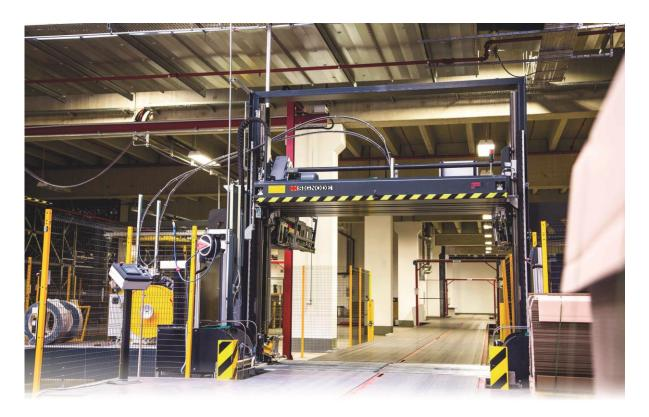
The GCU-2800 compression strapping press is equipped as standard with automatic top-edge protection applicators and bottom edge applicators to enable products to be compressed and strapped for storage and shipment to customers while providing optimum product protection and arrival condition at customers. The modular applicators seek and sense the pallet and the load and apply the protective strips before strapping.
