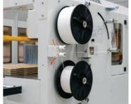
Automatic coil splicing Strap is automatically spliced from a second dispenser to provide up to 20,000m of strap for continuous production with zero downtime.
