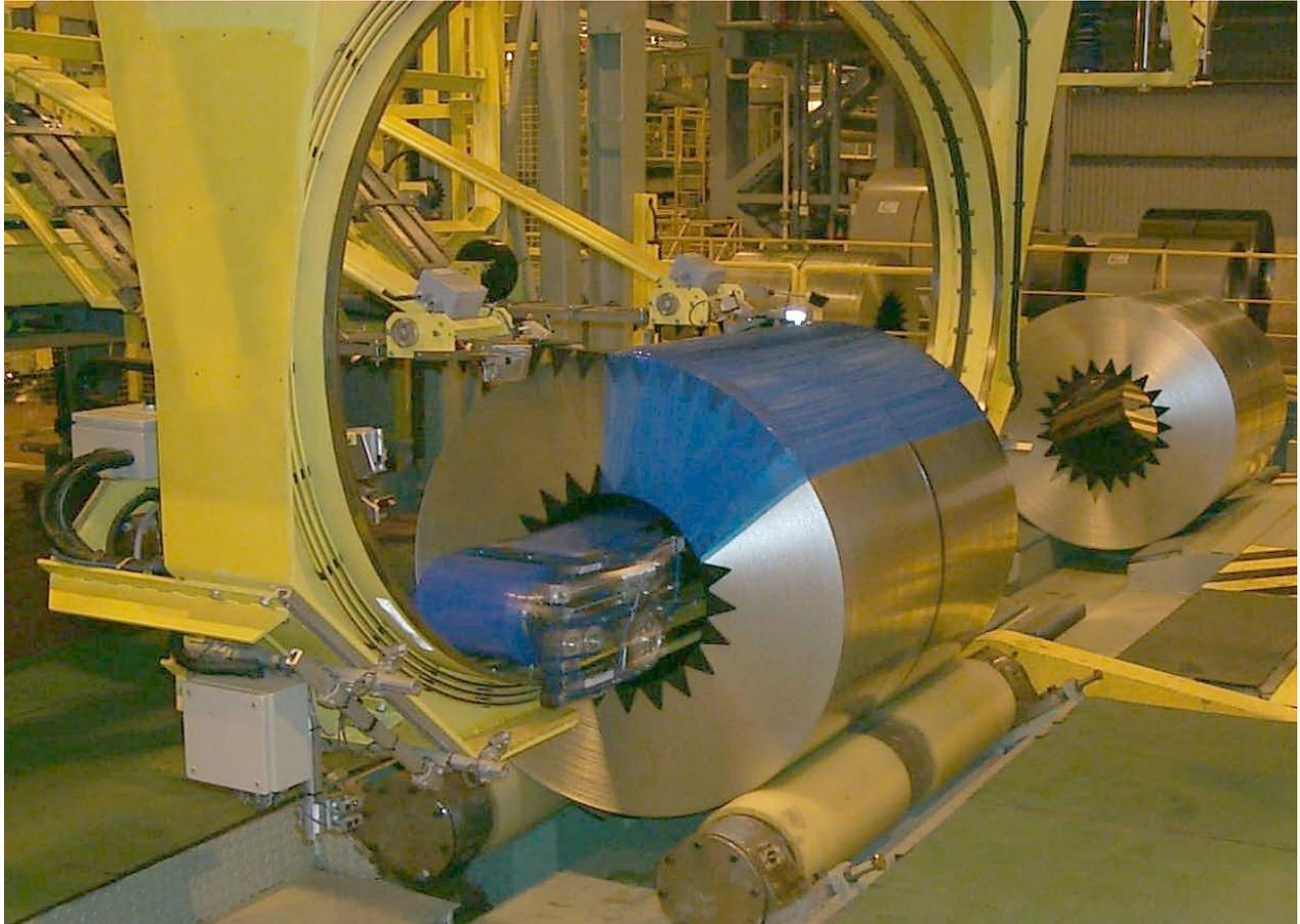
Designed for high performance through-the-eye wrapping of coils for the metals industry, the Coilmaster MK2 is available in a number of versions to suit most customers wrapping needs. The high speed carriage and the coil rotation in the machine determine the wrapping efficiency and coil protection levels. Shown here is the main film shuttle unit applying the outer film wrap over the automatically applied coil OD plastic heavy-duty edge-protection.
