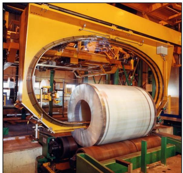
The powered film shuttle can apply a range of corrosion inhibiting films to the coil as well as protective films, strength films and also paper wrapping if needed. Depending on the options selected the machine is also able to apply coil outer edge plastic edge-protection and also plastic inner bore protection fully automatically during the wrapping process. A highly flexible packaging systems solution from Signode.
