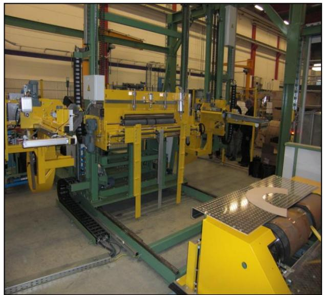
The Coilmaster Mark 2 can be equipped with automatic coil edge-protection applicators. The basic unit is composed of the jumbo coils of edge-protection on dispensers for each coil edge and applicator arms to find and feed the edge-protection onto the coil, during the film wrapping cycle.
