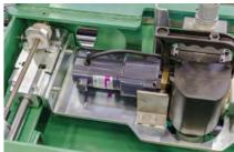
MH Modular sealing heads The modules use 9-12 mm machine grade PET strapping. The sealer unit requires maintenance every 100.000 cycles as does the feeder unit with few wearing parts.
