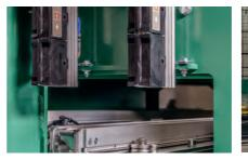
Indexing bayonet for flexibility With up to four chute systems and two bayonets the unit is extremely flexible to place strap on varying products very accurately.
