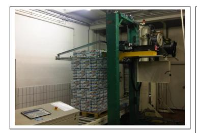
A Signode MH-H in operation in a frozen food storage and distribution centre. The unit here applies up to six straps to the loads depending upon the box dimensions. In order to accommodate a vast range of pallet loads the MH-H can apply up to eight straps per load from one of the eight standard, fully variable strapping programmes
