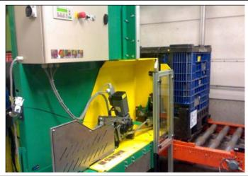
MH-VRB strapping shipping crates for world-wide shipment in an automotive spare parts warehouse
