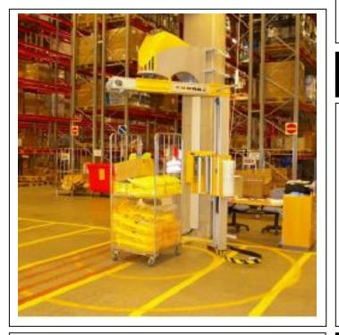
Variable, irregular and unstable loads being wrapped by a semi-automatic Cobra manually controlled crank-arm trolley wrapper. The small footprint of the crank-arm in park position enables easy fork truck access and with no turntable for wrapping no damage can be made to the equipment during the load handling operations,.
