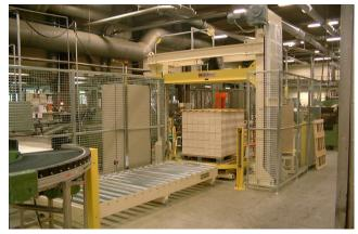
Paper Mill high productivity line with a SBM 4330 9mm strapping machine for A4 carton closure. Pallet load strapping and wrapping systems with end of line handling solutions can also be supplied.
