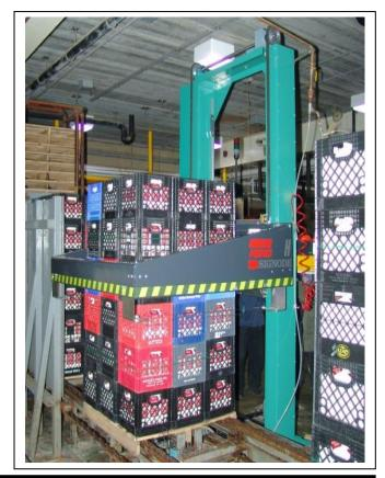
MH-H strapping crates for shipment in a dairy with 9mm PET strapping. An SBM 2330 strapping totes with 5mm PP in a pharmaceutical distribution centre
