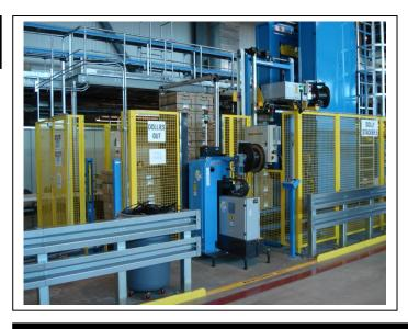
Horizontal and vertical Dolly MH strapping equipment at a FMCG Distribution centre
