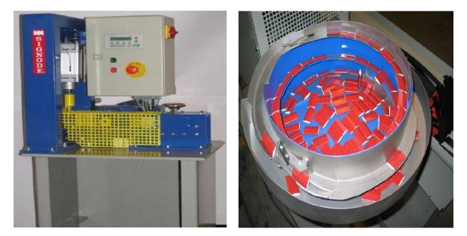
The main M-CTL robot is a highly compact, flexible unit which can cut straps to a pre-selected length and the number of straps can also be selected. Once the number of straps and their length has been entered into the system the unit works fully automatically. The unit can also be equipped with an optional seal feed and bender unit to produce pre-cut strap with push-type seals already applied to the straps
