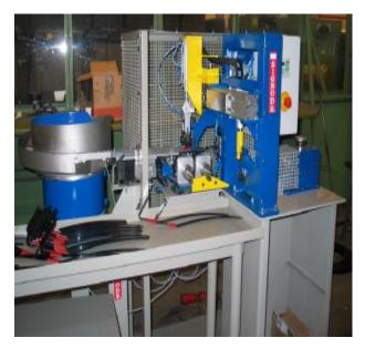
Optional seal feeder unit:- the seals are fed from the vibrating seal hopper into the seal guide magazine The robot gripper unit takes the metal seal and inserts it into strap bender unit before the strap is fed into the seal holder unit. This seal guide magazine ensures that all seals are correctly positioned and orientated before entering the seal gripper and strap bender unit
