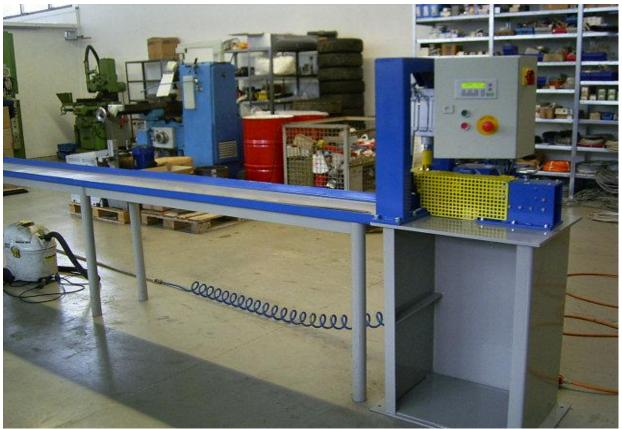
The MCTL, shown here with optional strap table, enables steel strapping or PET Polyester strapping to be cut to pre-determined lengths fully automatically. The unit is prepared for 16-32 mm steel strapping up to 1,6mm thick and PET strapping from 16 to 32mm width and a gauge of up to 1,3 mm
