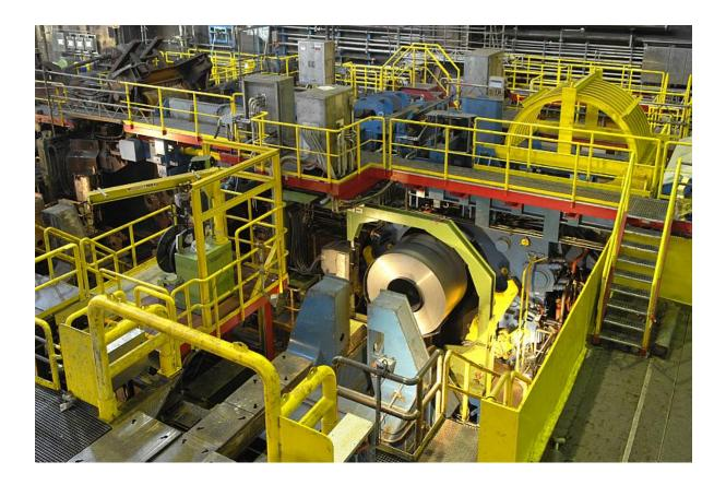
M410 CH3A here loacted on the exit of the rolling mill on a high speed, high throughput steel strapping application. The CH3A is designed to apply steel strapping to varying coil sizes & coil widths produced on the mill, to hot coils with coil surface temperatures of up to 750°C.
