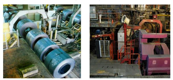
The M410 CH3A circumferential steel strapping machine can be equipped with a seal, seal less and also a spot weld version of the M410 steel strapping head for hot strip mill operations depending upon customer choice and application.
