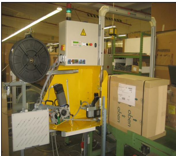
Fully automatic strapping of packaged kitchen cabinets The company reserves the right to make technical changes without prior notification
