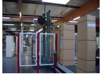
The MH-H horizontal model is able to strap varying load heights and sizes for high throughputs, and high machine uptime. The modular heads are easy to remove for preventative equipment servicing. The MH-H can apply up to eight straps per load from one of the eight standard, fully variable strapping programmes. The unit can thus accommodate almost all customers strapping pattern needs for very different furniture products.
