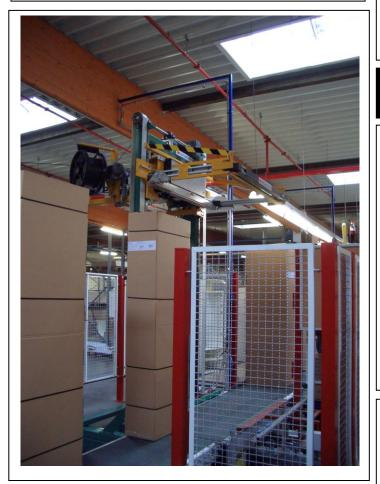
The MH-H horizontal machine works with both PP and PET strap to secure the packaging materials before shipment
