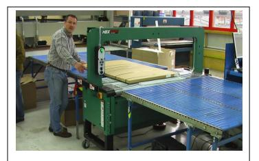
The SBM with its automatic strap feed and strap re-feed and jam-less technology is suited to the high demands in the furniture sector for machine ruggedness & uptime
