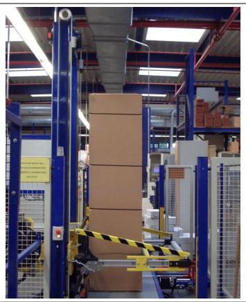
MH-H machines strapping cabinets on high-speed lines - up to 60 units per hour are possible
