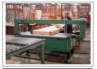
A 4300 unit strapping solid wooden doors and door skins for shipment with 12 mm PP strapping.
