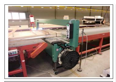
Above an 4330 large frame machine applies 9mm PP strap to flat-pack furniture to secure the paper packaging materials to protect the product.
