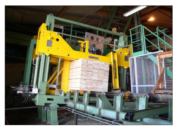
Models shown as a Tandem, high throughput HD-LP press station with an optional service platform. The side and top compression arms are free-floating for optimum load compression and stabilization.
